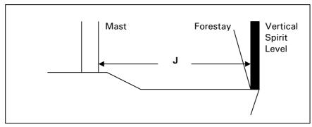
**FL** is measured with the mast stepped and chocked at deck level, standing rigging tensioned, and backstay/runners hand tight. If the forestay is adjustable (either while racing or at any other time) it must be set to the maximum length that will be used while racing. As with P, this should be done on a day with light winds to avoid inaccuracy due to wind effects on the tape measure.
