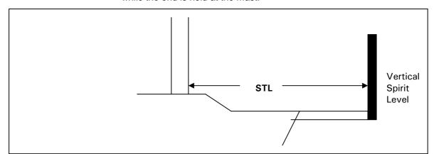
Spinnaker tack point on deck: As for bowsprit, but with the spirit level positioned at the spinnaker tack point on deck.
